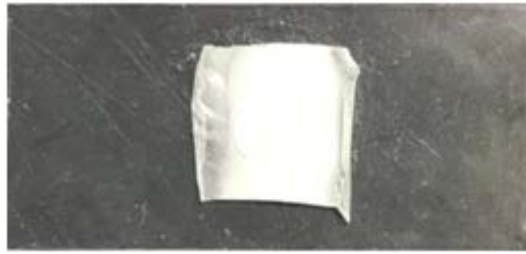
Figure 4. Cut-off membrane of PLA manufactured by electrospinning.
