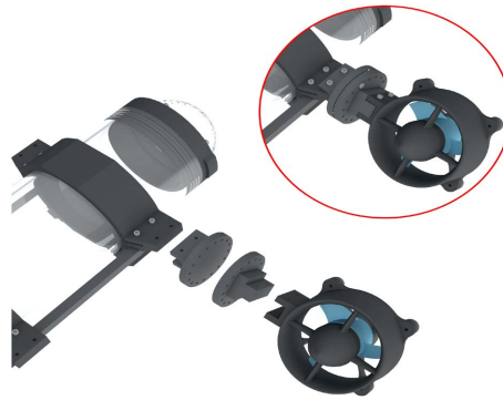
Figure 6. A design of an adapter which can have five possible orientations.
