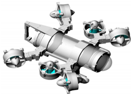
Figure 11. This is the design part of the micro-robot, which has six thrusters.
