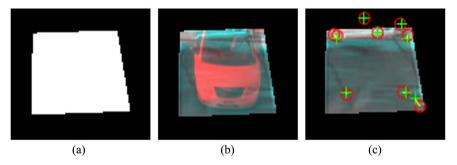
**Figure 5.** MATLAB SURF detector process. (a) Polygon drawn for a parking space; (b) Same polygon with a vehicle; (c) Same polygon for the empty space, where points of interest from the base image are detected.
