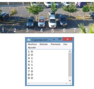
**Figure 8.** Parking spots with and without vehicles, and the respective MATLAB output represented with 0 (empty/available space) and 1 (taken space).
