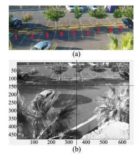
**Figure 4.** Base image used for the prototype. (a) Numbered parking spaces; (b) MATLAB delimitation of the parking space.
