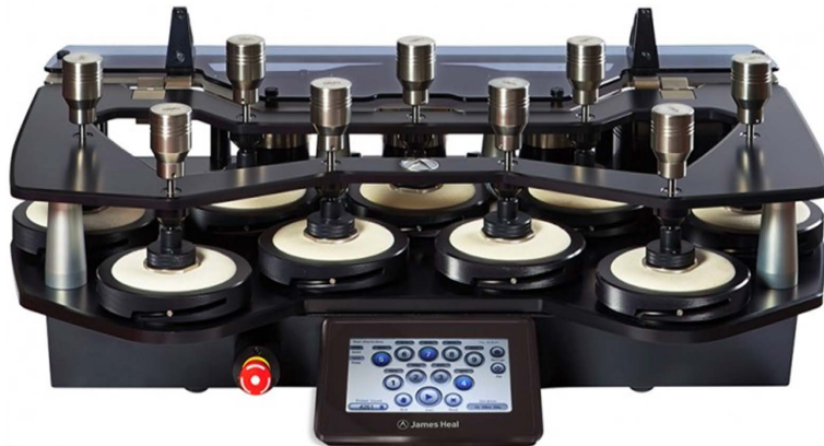
Figure 4. Martindale pilling and abrasion tester.
