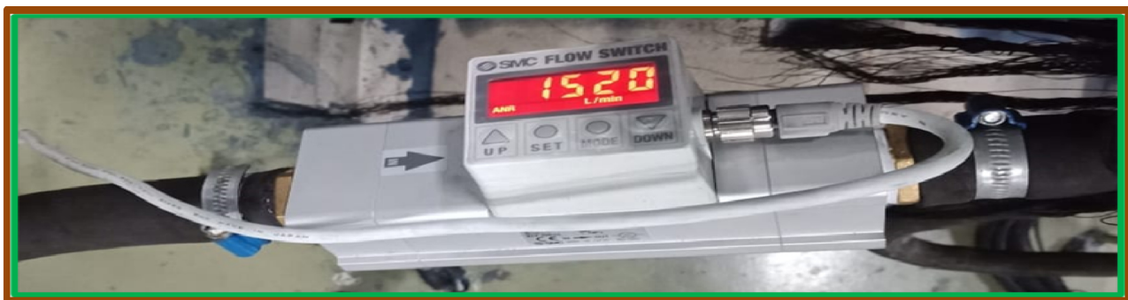
Figure 4. CFM meter for air consumption measurement.
