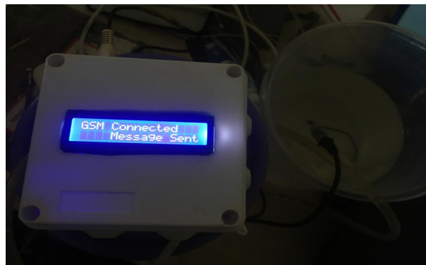
Figure 3. Indication of a GSM module being connected.
