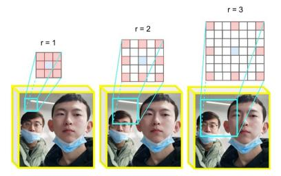
**Figure 4.** The pixel points are involved in the computation of the convolution kernel when the dilation factor is 1, 2 and 3.
