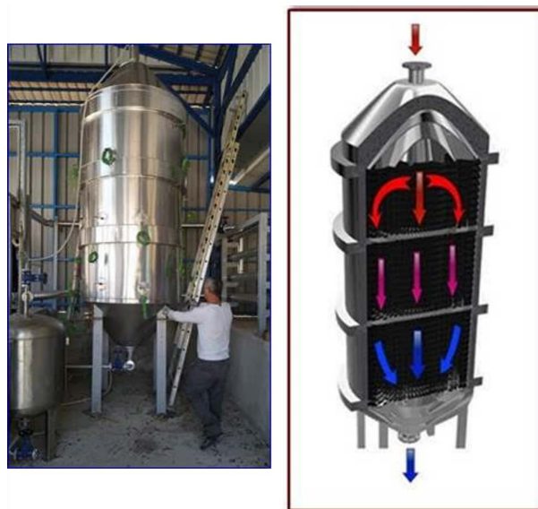
Figure 5. The experimental 2 m 3 magnetite TES tank (left) and internal structural details and flow configuration during charging (right).
