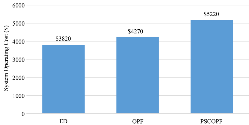
Figure 8. Total system operating cost for ED, OPF and PSCOPF.
