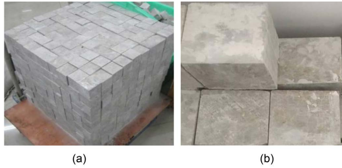
Figure 4. Photos of different rock blocks. (a) 5 cm × 5 cm × 5 cm rock block; (b) 10 cm × 10 cm × 10 cm rock block.
