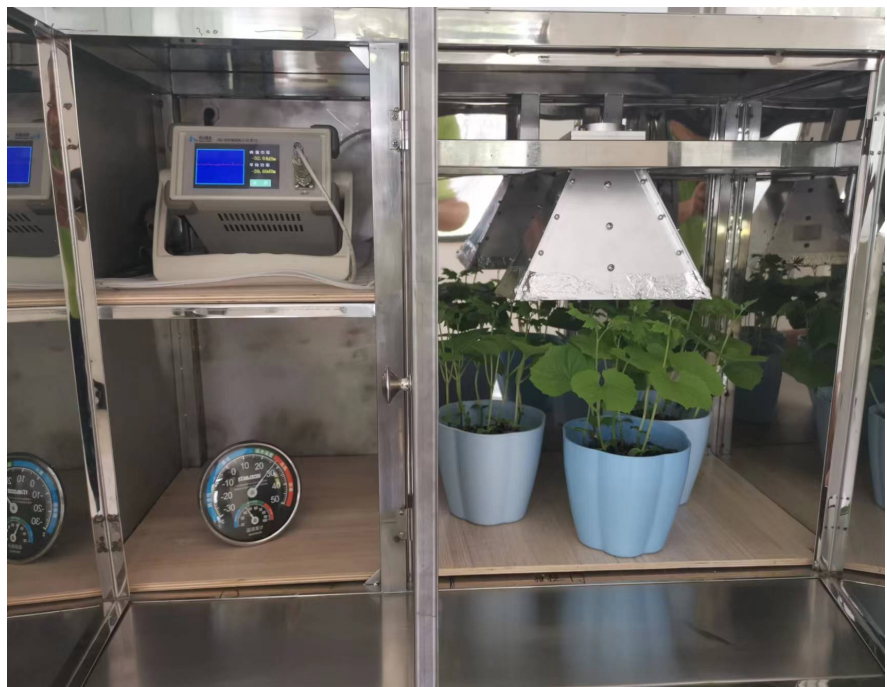
Figure 6. The staff are using the biological radiation signal power detector to detect the radiation signal power of plants, and use the data to judge the growth state of plants.
