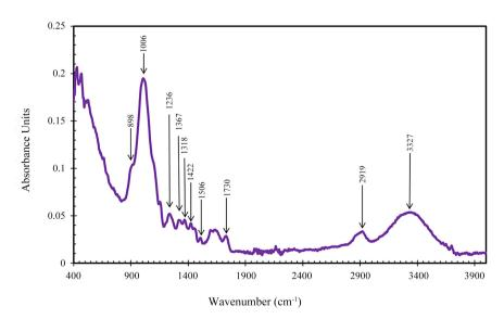
Figure 3. ATR-FTIR spectrum of CL fibers.
