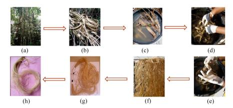
**Figure 2.** Extraction process of CL fibers. (a) CL plants selected, (b) CL bark, (c) Submerged CL bark, (d) Washing of CL bark after 4 weeks of soaking, (e) Rinsing of CL fibre bundle, (f) Dried CL fibre bundle (g), CL fiber bundles, (h) CL fiber.
