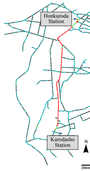
Figure 12. Route obtained adopting Dijkstra's algorithm between Kurodasho Station and Honkuroda Station.
