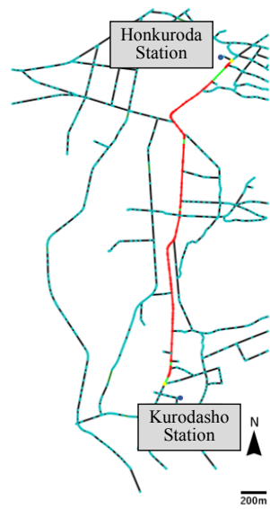
Figure 13. Route obtained adopting the improved ACO between Kurodasho Station and Honkuroda Station.
