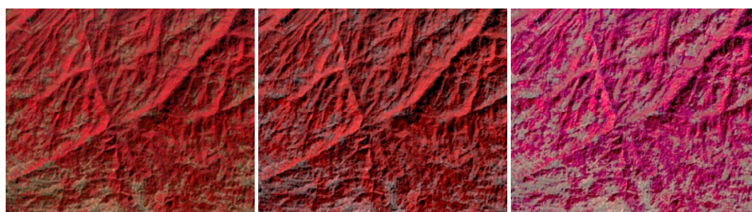
Figure 3. (a) Raw satellite imagery, (b) Atmospherically corrected imagery, (c) Topographically and atmospherically corrected imagery respectively.
