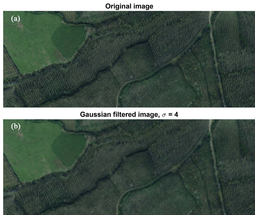
Figure 3. (a) Original image; (b) Gaussian filtered image obtained with filter size of 17 \times 17 and \sigma of 4
