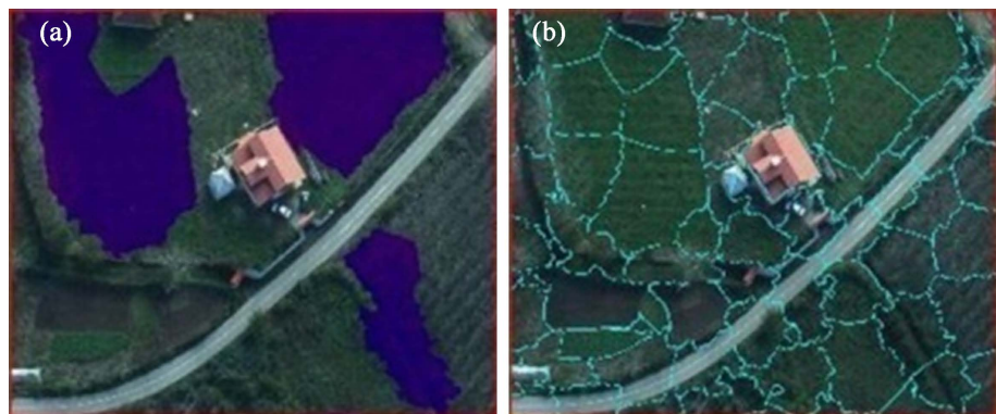
Figure 8. (a) Separated highly vegetated land cover (colored part in the right side image) resulted from applying an NDVI threshold that was overlaid on the RGB image. (b) is related to the corresponding segmented RGB image.
