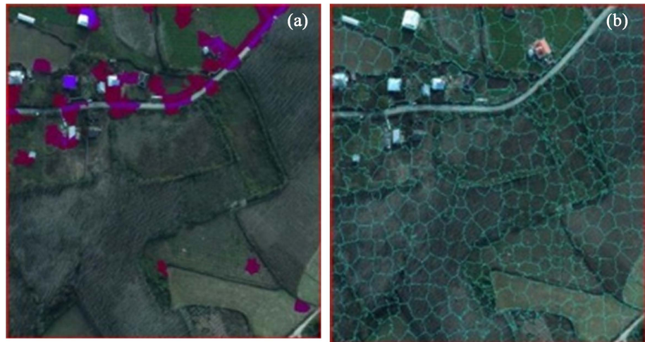
Figure 7. (a) Separated built-ups and bare soil (colored part in the right side image) resulted from applying function 9 threshold was overlaid on the RGB image. (b) is related to the corresponding segmented RGB image.
