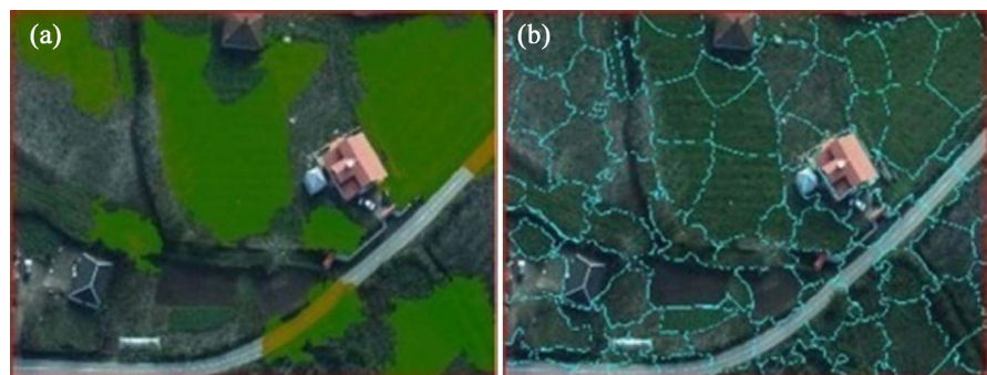
Figure 6. (a) Separated green farms and gardens (colored part in the right side image) resulted from applying NGI threshold that was overlaid on the RGB image. (b) is related to the corresponding segmented RGB image.
