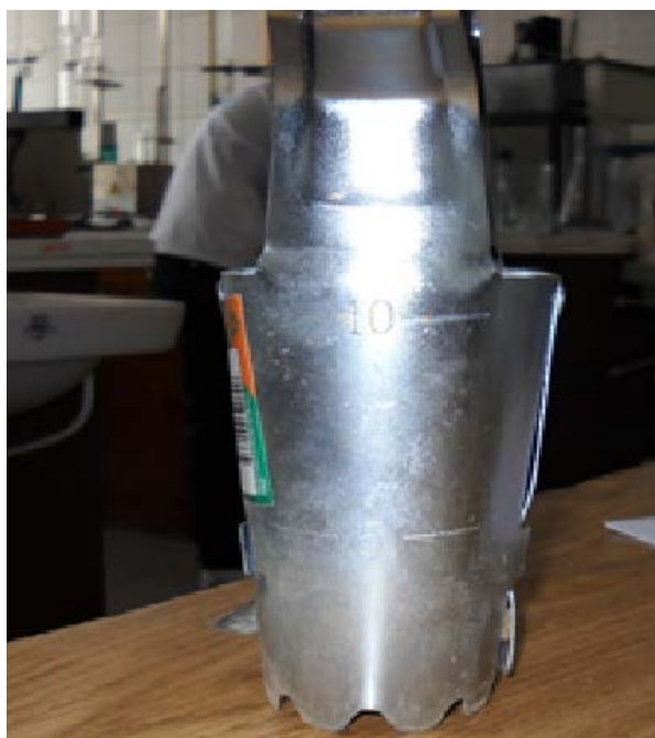
Figure 1. Soil sampling device (device made by author).
