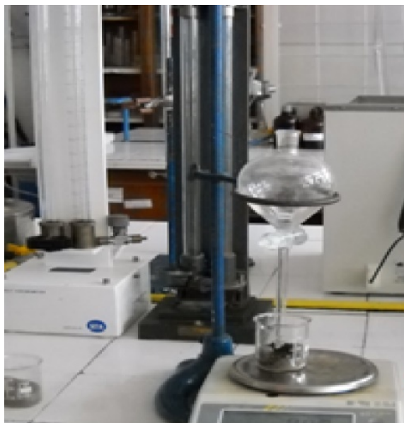
Figure 2. Plant for the study of soil adsorption of pollutants (device made by author).
