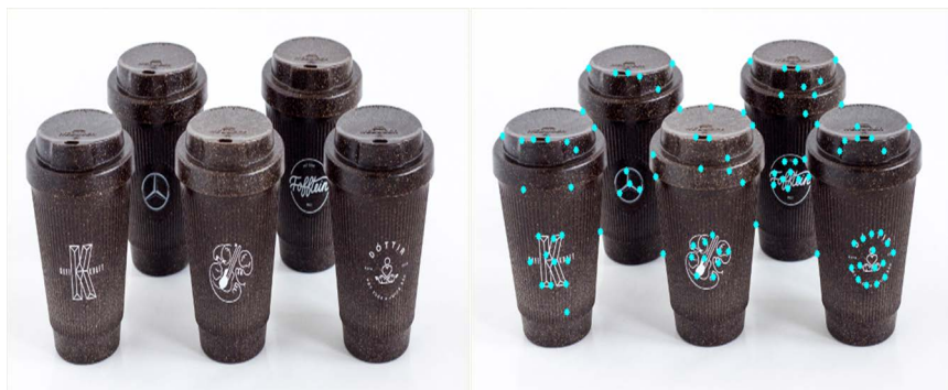
Figure 4. Grasping detection using corner detection. The left image is the original image which is the data, and the right one shows the result of corner detection using python.
