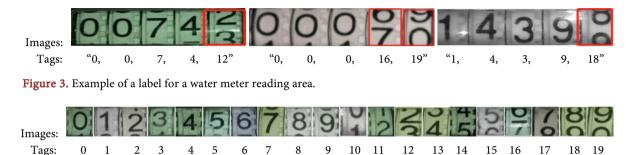
Figure 4. Example of a single number and label in a water meter image dataset.
