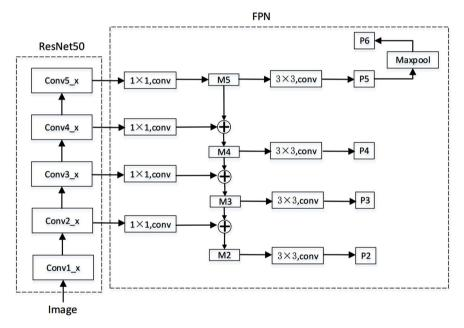
Figure 7. ResNet50 combined with FPN for feature extraction network.
