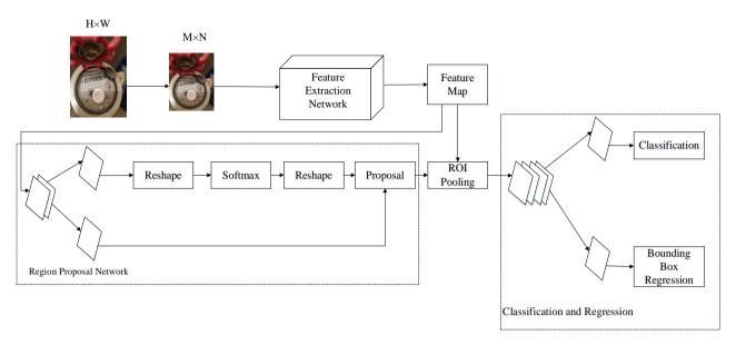
Figure 6. Faster-RCNN network structure.
