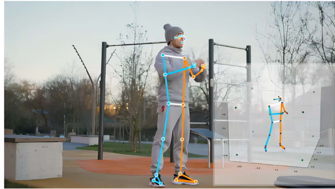
Figure 1. Mediapipe Pose's position detection of 33 posture joints.
