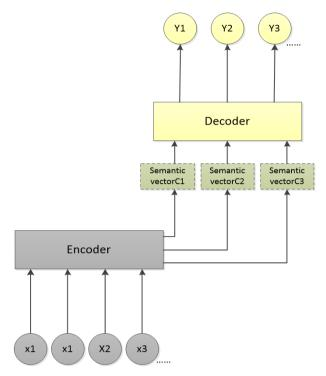
Figure 4. Seq2seq model architecture with Attention mechanism.
