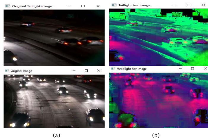
Figure 7. (a) Original images and (b) HSV color space of the original images.
