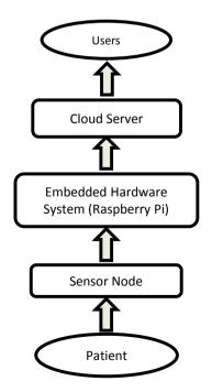
Figure 3. Proposed model for IoT cloud based healthcare system.
