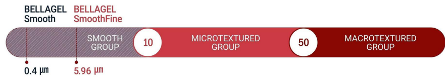
Figure 1. The BellaGel® SmoothFine based on the international organization for standardization classification. The BellaGel® SmoothFine is equipped with a refined, smooth surface with a roughness of 5.96 mm, which is a different feature from traditional smooth surface.
