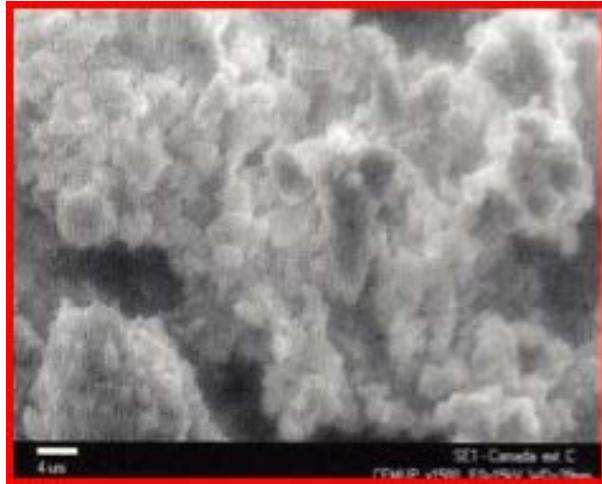
Figure 9. Mineralization on MES membrane after 7 days of immersion in synthetic plasma, MEV 1500×.
