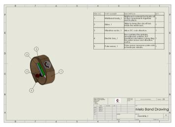
Figure 3. Bill of Materials for the Device.
