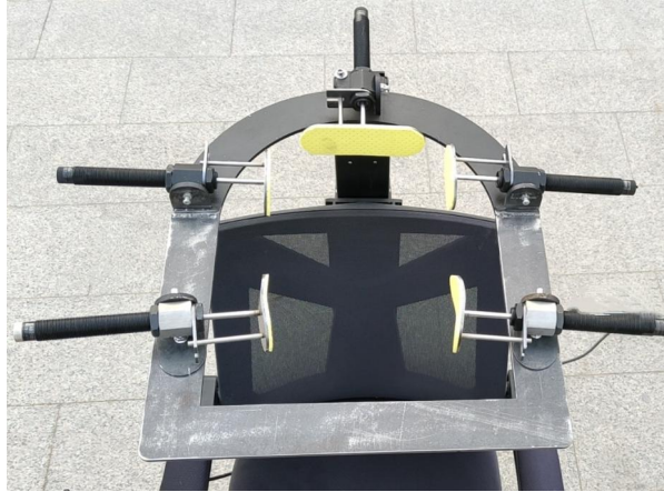
Figure 7. Anti resistance head ring of cervical vertebra self training instrument.
