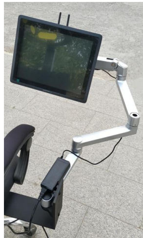
Figure 8. Cervical vertebra self training instrument Touch control all-in-one machine and support arm.
