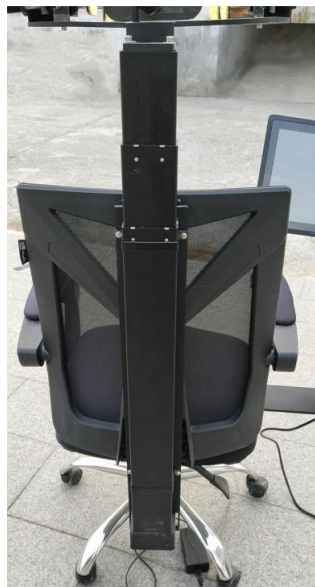
Figure 9. Head ring automatic regulating system.
