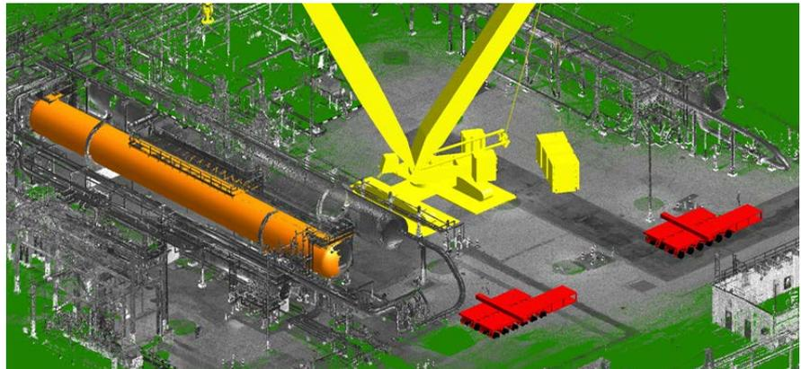
**Figure 2.** Existing vessel, crane, and SPMT are depicted as 3D models.
