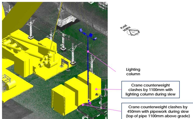
**Figure 7.** Clash C4—Crane’s counterweights clash with the lighting pole during the slew.
