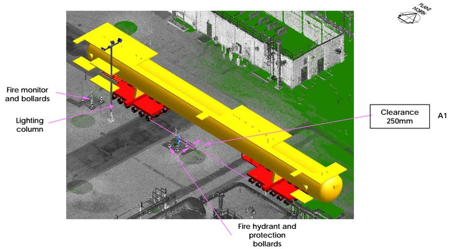
**Figure 8.** Clash A1 – Fire monitor and hydrant.
