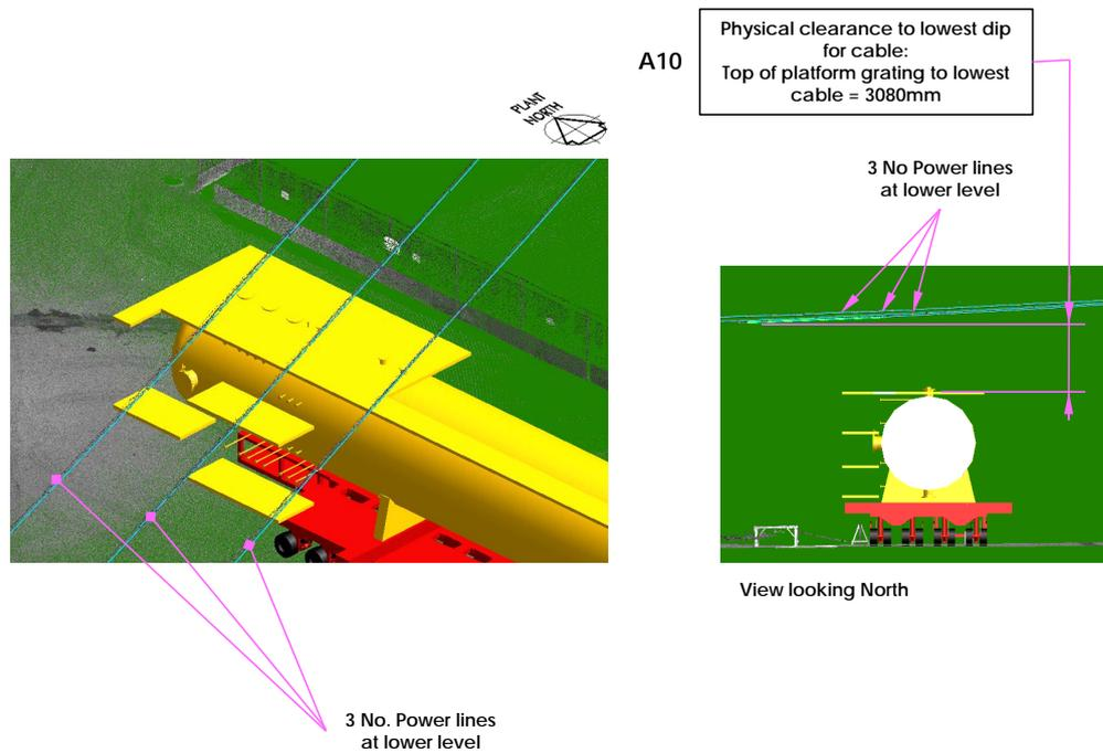
**Figure 9.** Clash A10 – Overhead power lines.
