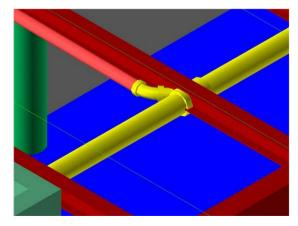
Figure 3. A typical hard clash between piping and structural models.
