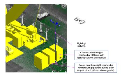
Figure 7. Clash C4—Crane's counterweights clash with the lighting pole during the slew.
