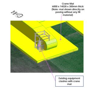
Figure 6. Clash C3—Crane clashes with existing equipment.
