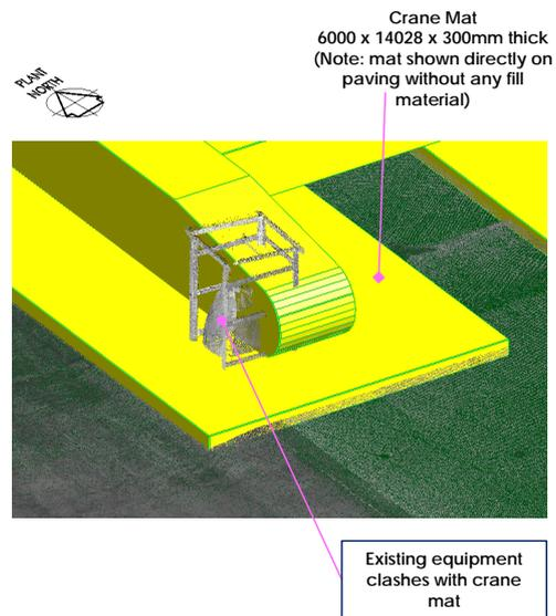
**Figure 6.** Clash C3—Crane clashes with existing equipment.
