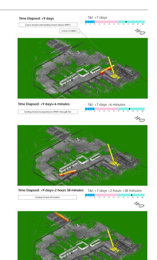
Figure 10. Crane set up and vessel movement against the timeline.
