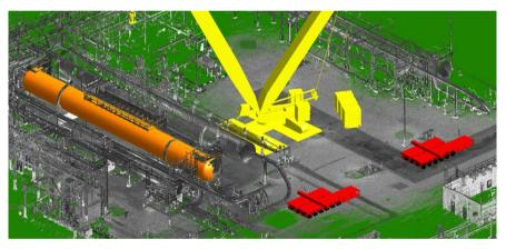
Figure 2. Existing vessel, crane, and SPMT are depicted as 3D models.
