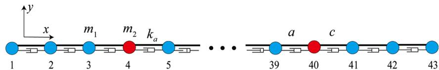
Figure 14. Lattice chain model with damping.
