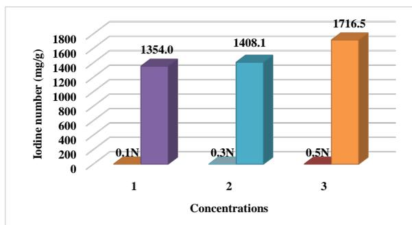
**Figure 6.** Iodine value of powdered activated coals to the different concentrations at 400°C.
