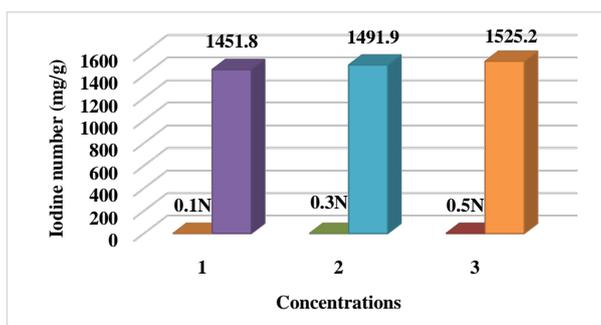
**Figure 8.** Iodine value of grain activated coals to the different concentrations at 400°C.
