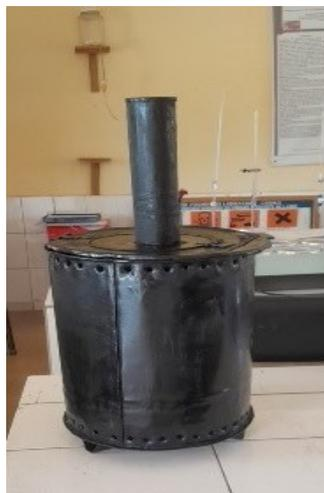
**Figure 3.** Photos of the carbonizer.
