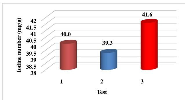
Figure 5. Iodine value of non-activated coal.
