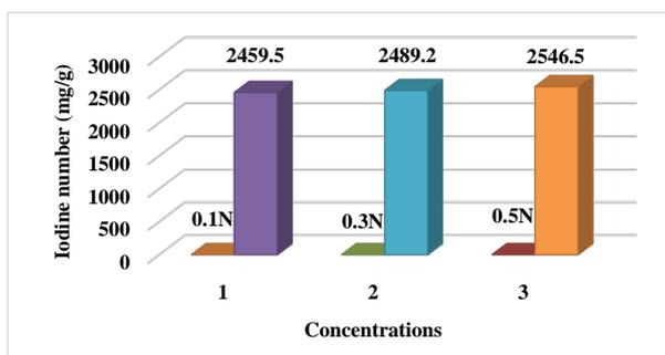
**Figure 7.** Iodine value of powdered activated coals to the different concentrations at 700°C.
