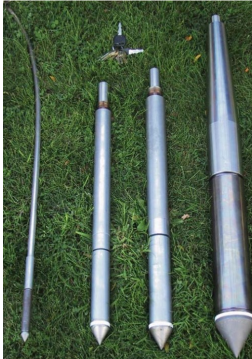
Figure 3. 5 cm 2 , 10 cm 2 , 15 cm 2 and 40 cm 2 penetrometers [8].
