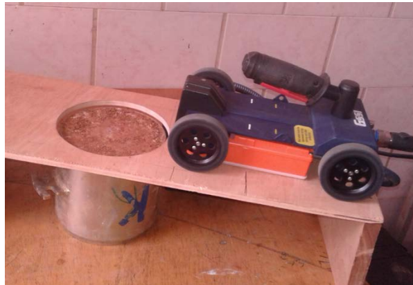
Figure 2. Data acquisition device, showing the laterite soil sample in the Proctor mold and the 1.6 GHz antenna.
