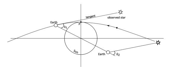
**Figure A3.** The star is observed at an angle  $\delta_1$  at a different position on the sky than its "true" position  $\delta_2$ , measured half a year later. For illustrational purposes the bending is hugely exaggerated. A more detailed and on-scale figure can be found in [3].
