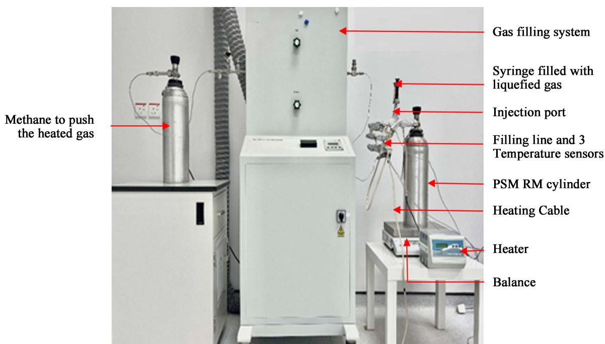
Figure 2. Injection system of liquefied i-pentane, n-pentane and n-hexane natural gas components.
