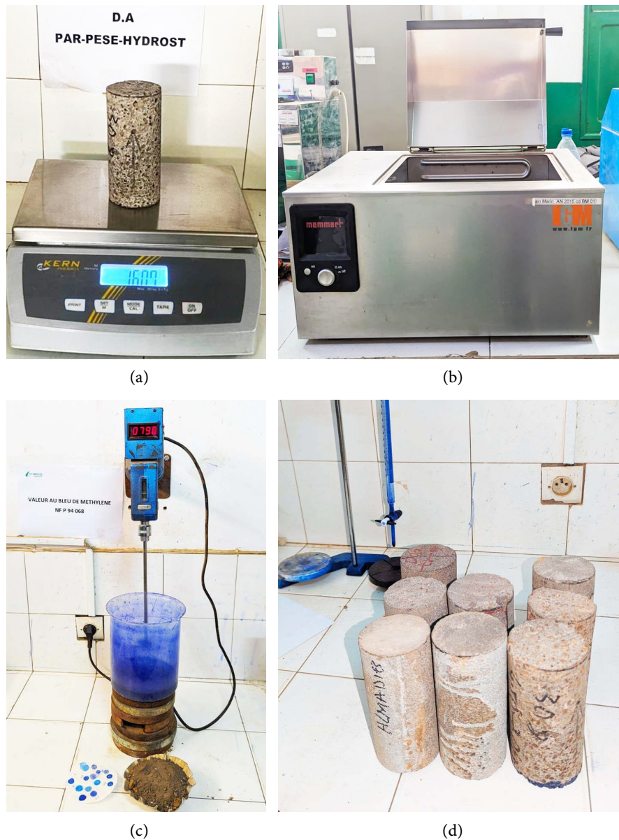
Figure 2. Different methodological phases ((a) dry density measurement, (b) marine bath for saturation, (c) methylene blue value measurement device, (d) cylindrical rock samples for simple compression).
