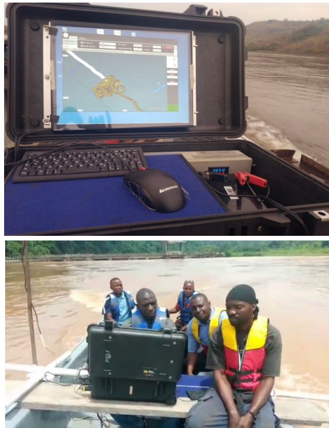
Figure 4. Echosounder-GPS interface, bathymetric survey and bathymetric team in the Shongo basin.
