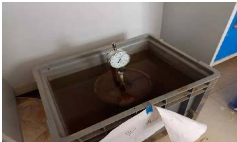
Figure 1. The preparation of the soil sample in immersion for 4 days.
