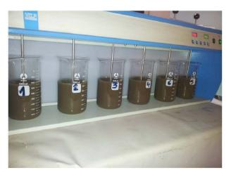
Figure 2. Jar-test device.
