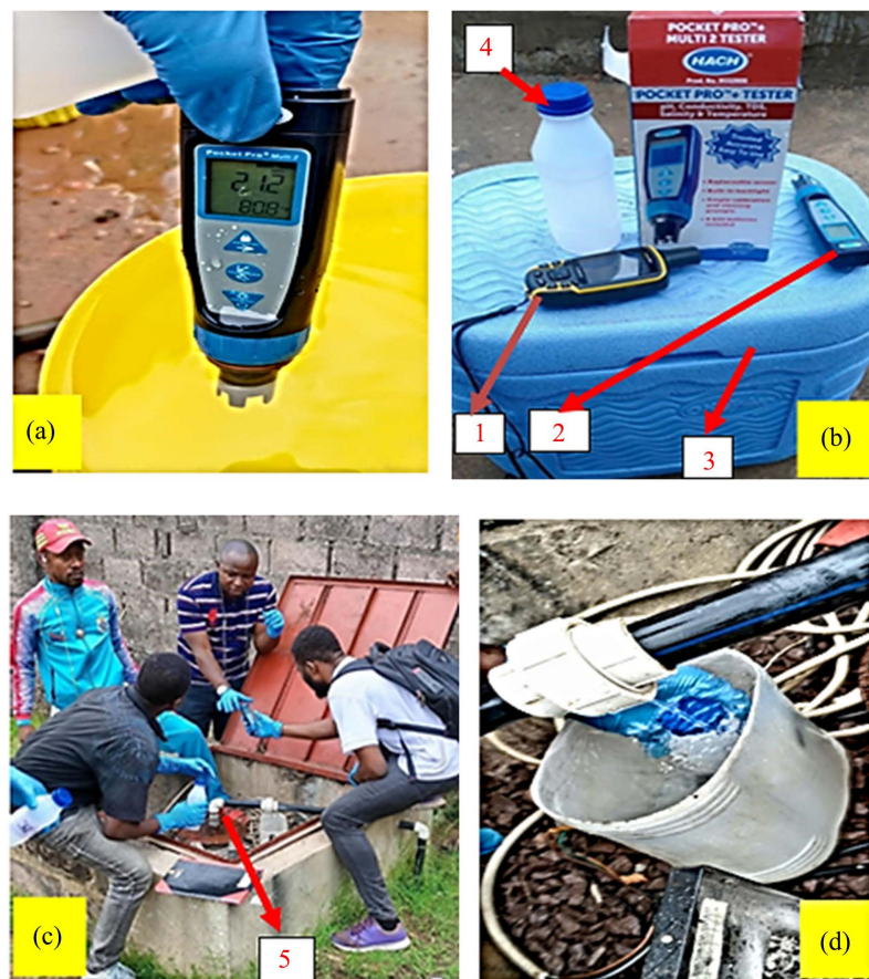
Figure 2. (a): In-situ sampling of pH, T°, TDS, Salinity, electrical conductivity with the multi-parameter probe; (b): Equipment used to collect and preserve samples: a GPS (1), multi-parameter probe (2), a cooler (3), bottle (4); (c): Sampling of the water which leaves the aquifer after pumping before reaching the cistern at the borehole flange level (5); (d): Sampling of water leaving the aquifer after pumping.
