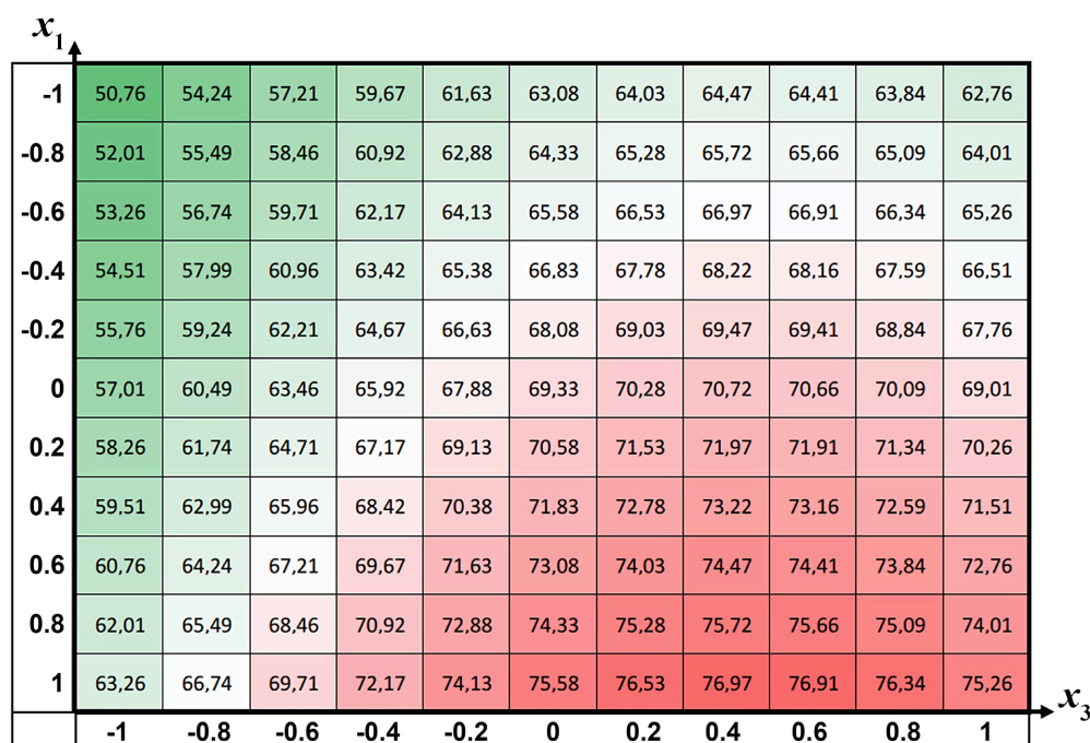
Figure 2. Graph of the dependence of the number of rotations of the saw drum on the angle of inclination of the guide.
