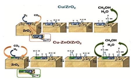
**Figure 7.** Heterogeneous catalytic process for conversion of  $CO_2$  to methanol using Cu/ZrO<sub>2</sub> and Cu-ZnO/ZrO<sub>2</sub> (adopted from [20]).
