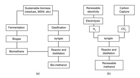
**Figure 1.** (a) Bio-methanol production processes (b) Renewable methanol production processes from different feedstocks. Reproduced from: [5].
