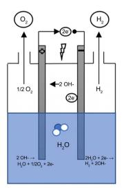
**Figure 4.** An electrolyzer (Reproduced from [16]).
