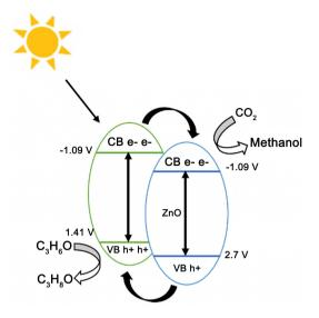
**Figure 5.** Schematic of photocatalytic reduction of CO<sub>2</sub> system [24].
