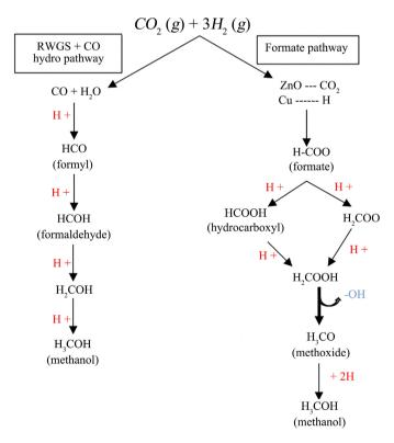
**Figure 8.** Pathways of methanol production from CO<sub>2</sub> hydrogenation over Cu-based catalysts (Reproduced from [1]).
