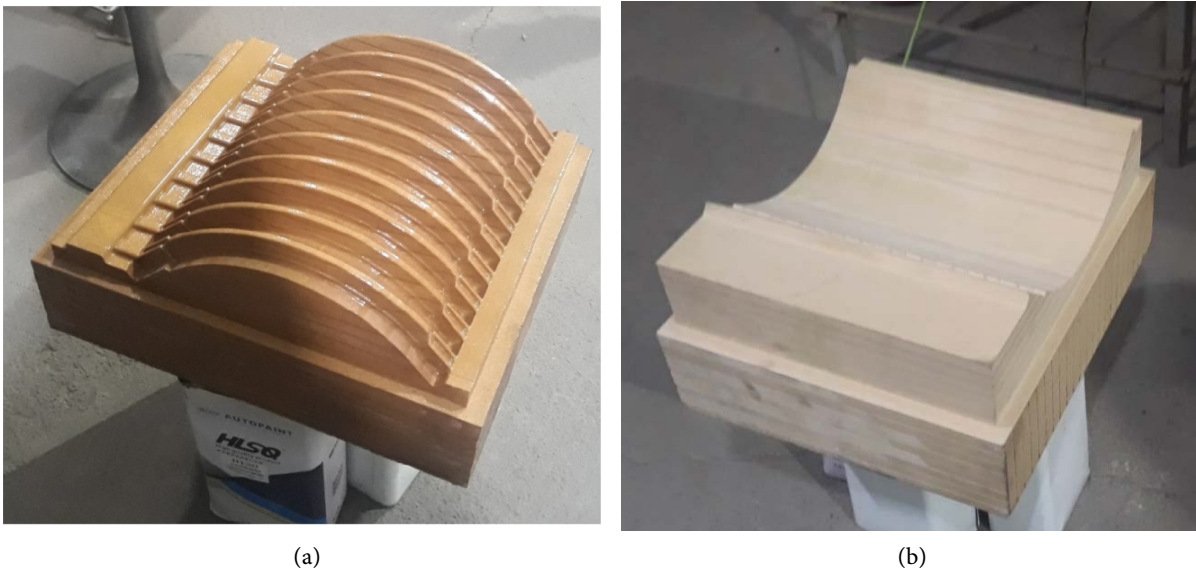
Figure 2. Casting mold from MDF. (a) Stamping punch; (b) Former block.
