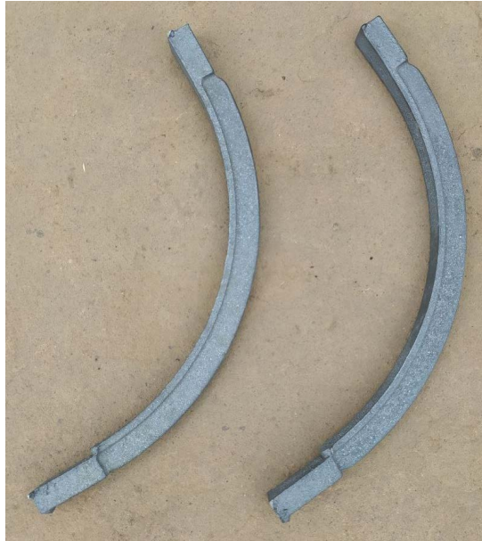
Figure 5. Ready rib by aluminum mold.
