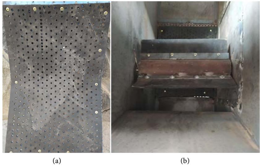
**Figure 7.** Working bodies of the improved stone trap device. (a) Mesh surface; (b) elastic-coated, bladed drum.
