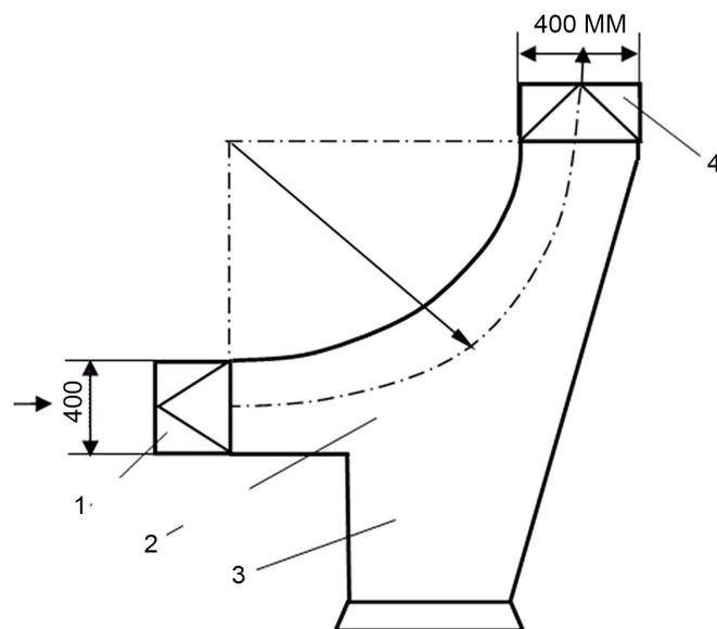
**Figure 4.** Radial stone catcher. 1-inlet pipe, 2-separation chamber, 3-pocket, 4-outlet pipe.
