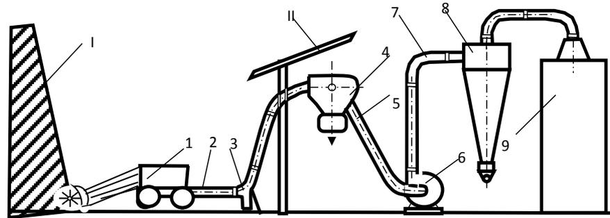
**Figure 3.** Air transport device in ginneries. 1-mechanical cotton transfer equipment for pipe; 2-working tube; 3-stone catcher; 4-separator; 5-suction air duct; 6-fan; 7-exhaust air duct; 8-cyclone; 9-dust collector; (I-riot, II-production workshop).
