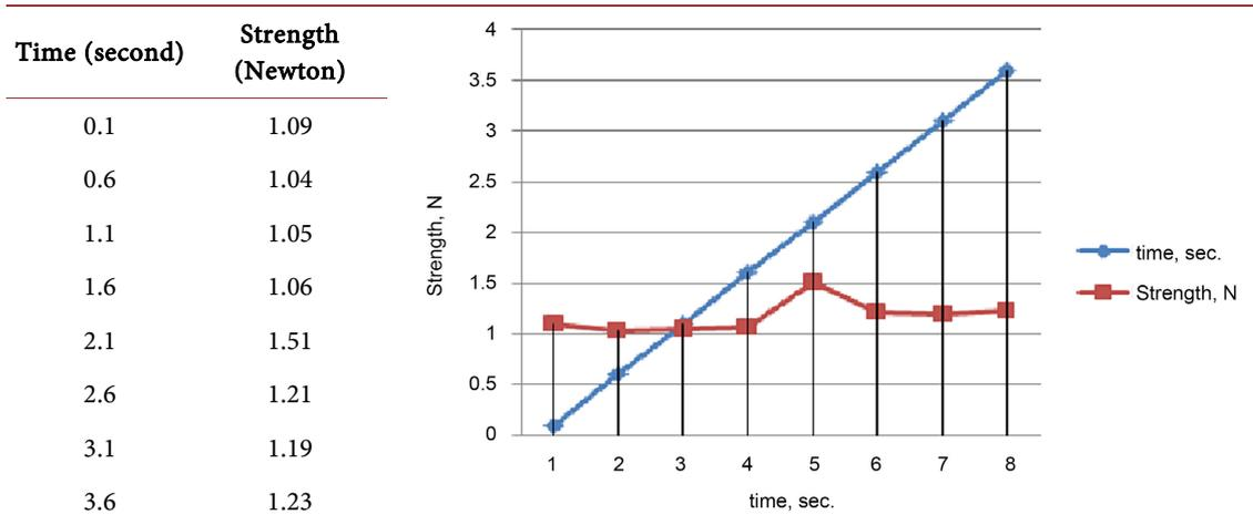
Figure 9. Results of experiments on the determination of the impact force in an improved stone catcher device.
