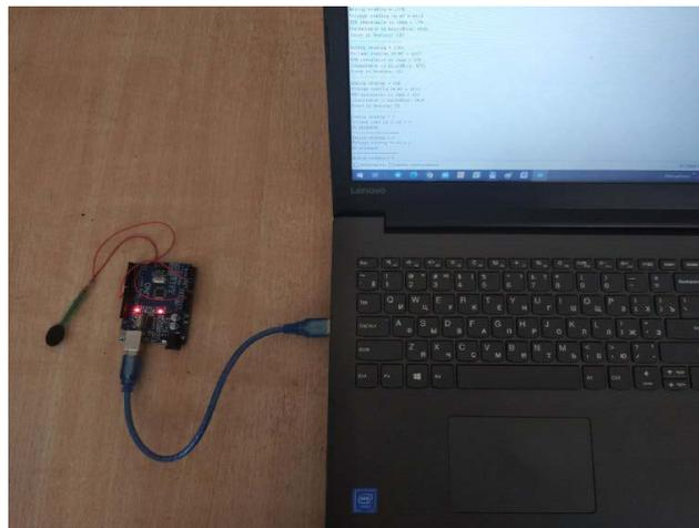
**Figure 8.** A computer-generated view of the FSR sensor that detects the force of an impact.
