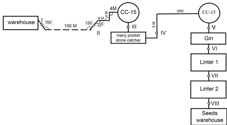
Figure 1. Scheme of raw cotton processing in ginneries. I-VIII sample points.
