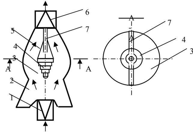
**Figure 5.** Vertical stone chatcher. 1-inlet pipe; 2-pockets; 3-separation chamber; 4-return step wall; 5-Router; 6-outlet pipe; 7-plate.
