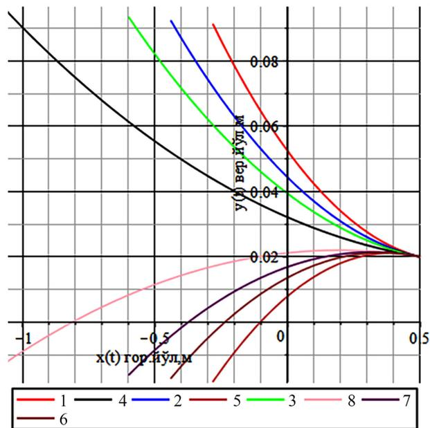
Figure 10. Laws after impact movement of cotton and heavy mixtures entering the improved stone trapping chamber. On the graphs, the coefficient of high-speed return of the receiving and softening mesh of the curvilinear plate of the impact force is equal to  $n = 0.5; 0.6; 0.7; 1$ ; Graphs 1 - 4 are for the cotton portion and graphs 5 - 8 are for heavy mixes.
