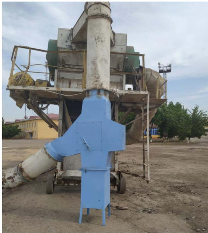
**Figure 6.** Improved stone trap device.
