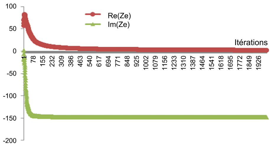
Figure 4. Convergence of the input impedance of the study structure as a function of iterations. (Number of iterations: 2000).
