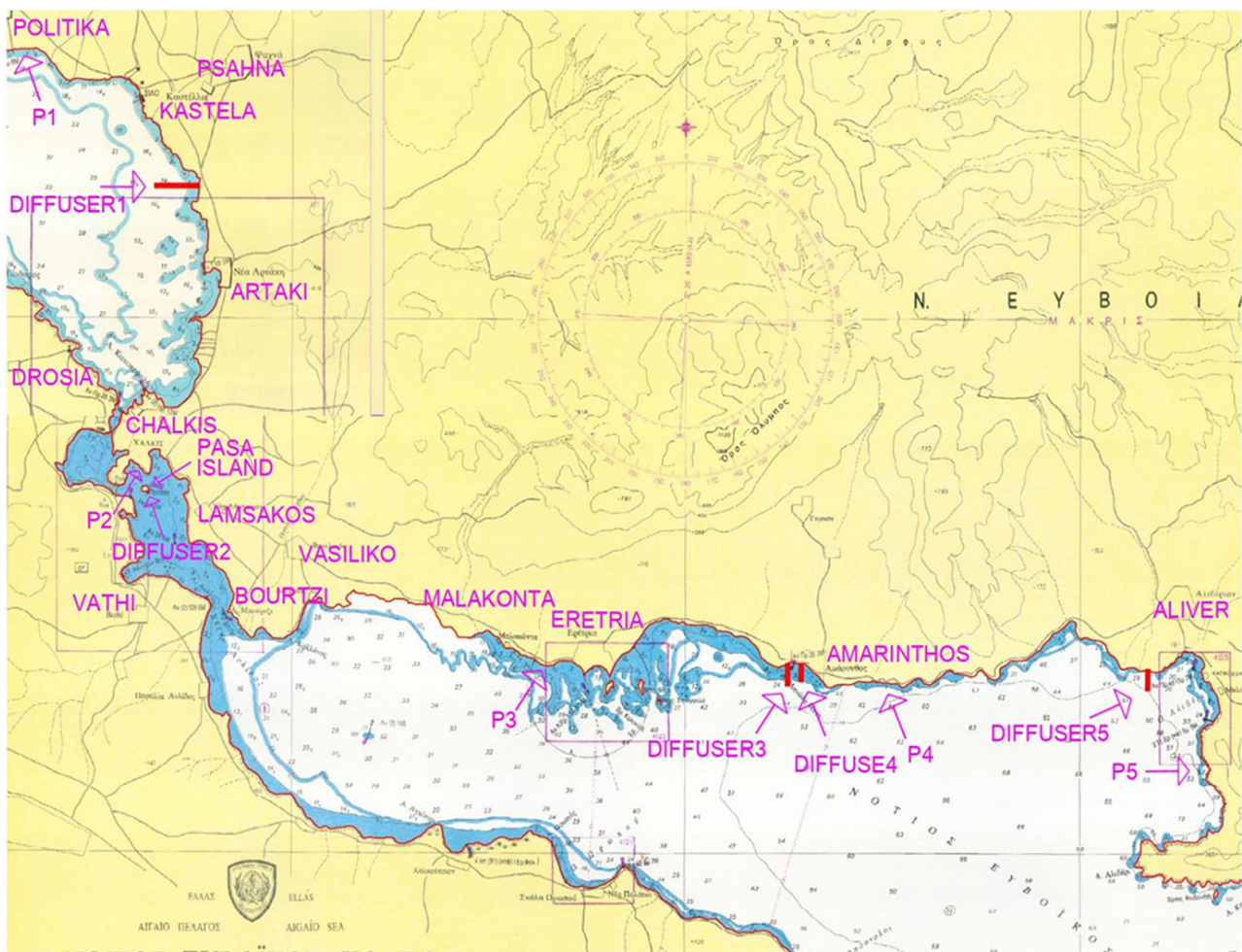
Figure 6. Visual representation depicting the positions of underwater urban wastewater disposal pipelines within the Euboean Gulf, along with the identification of designated control sites situated in the coastal areas, illustrated on a 1:100.000 scale map.
