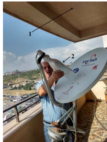
Figure 2. Calibration facilities of ArtAr-HDF in the city of Yerevan 1—Concrete ceiling (Gray Body) with an emissivity of \sim 0.95 , 2—Black Body with an emissivity of \sim 0.974 .
