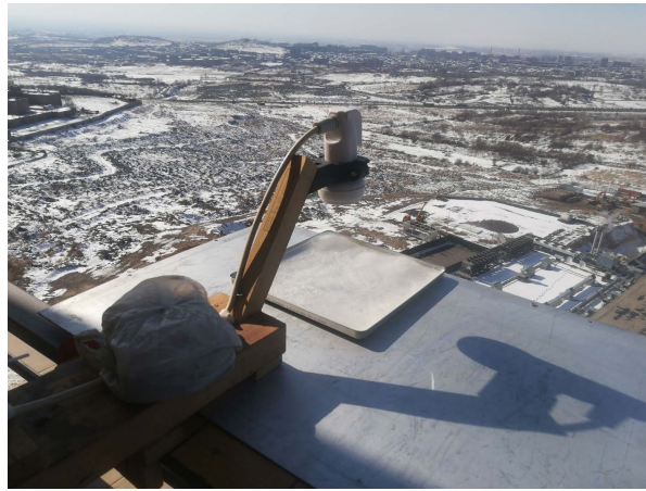
Figure 10. An experiment with a duralumin tray with frozen thin (8 mm) ice layer on a duralumin sheet.
