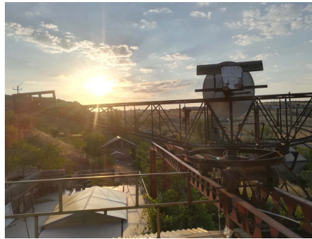
Figure 4. Ku-band, 100 cm dish antenna and LNB of ArtAr-HDF are installed on mechanical scanner at a height of 10 m from the ground in experimental site of ECOSERV ROC Co. Ltd. near the Village of Ujan and directed East to measure sky emission and solar emission during sunrise.
