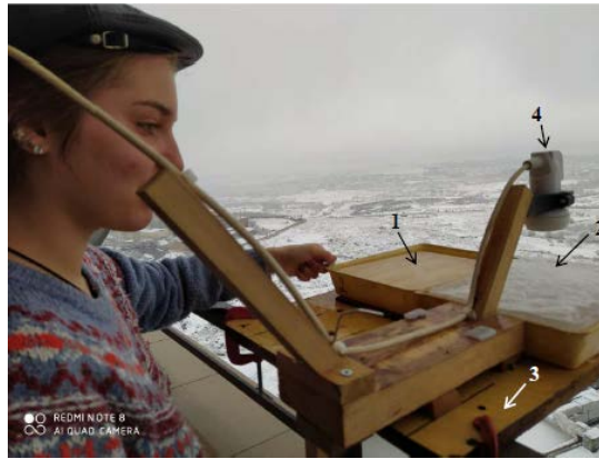
Figure 8. Experiments with water and ice in plastic trays placed on a wooden stand. 1—A plastic tray with water of \sim 4 cm, 2—A plastic tray with rectangular rough ice layer of \sim 4.5 cm at \sim -4^{\circ}\text{C} , 3—A wooden stand, 4—LNB.
