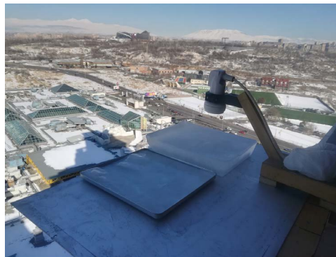
Figure 12. An experiment with 8 mm thin and 4.5 cm thick ice layers on a duralumin sheet.
