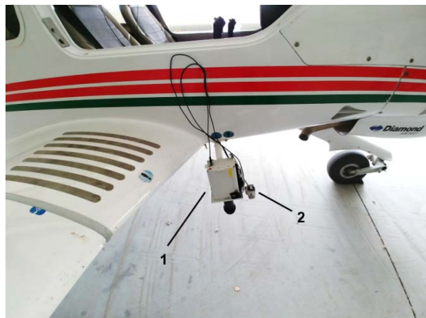
Figure 2. The FSR-02 spectrometer coupled with a survey camera installed on board the Diamond DA40NG aircraft: 1—FSR-02 spectrometer; 2—survey camera.
