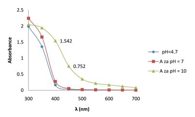
**Figure 4.** UV-Vis spectrum for different solutions of silver nanoparticles synthesized from orange peel extract as a function of pH value at a concentration of 0.1 mM AgNO<sub>3</sub>.
