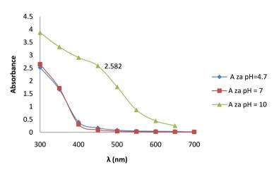
**Figure 2.** UV-Vis spectrum for different solutions of silver nanoparticles synthesized from orange peel extract as a function of pH value at a concentration of 1mM AgNO<sub>3</sub>.
