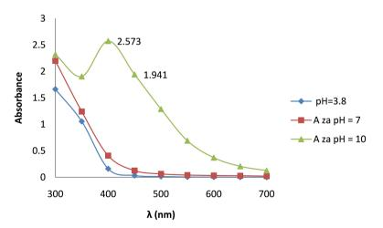
**Figure 5.** UV-Vis spectrum for different solutions of silver nanoparticles synthesized from lemon peel extract as a function of pH value at a concentration of 0.5 mM AgNO<sub>3</sub>.
