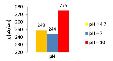
**Figure 3.** Conductivity of solutions of silver nanoparticles synthesized from orange peel extract and 1 mM AgNO<sub>3</sub> as a function of pH.
