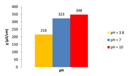
**Figure 6.** Conductivity vs pH solution of AgNPs synthesized from lemon peel extract and 0.5 mM AgNO<sub>3</sub>.
