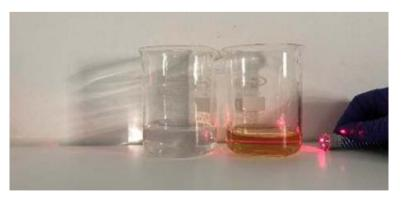
**Figure 7.** Comparison of the passage of laser light in relation to distilled water (left) and a solution of silver nanoparticles (right).
