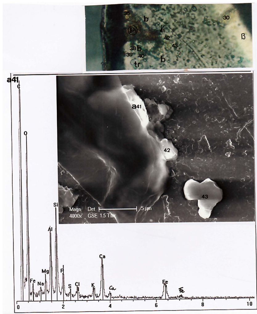
Figure 6. The a41 particle. Above photograph: optical view (1200 \times ) of the left part of the low A area, showing the a41 particle (arrow point). P1 is a triangular fold of PVC plastic in this area part (B is the right border of the A area). Below photograph: SEM1 photograph (4000 \times ) in GSE, showing the emerging part of the a41 particle (a42 is a glass and a43 a trilobed calcium carbonate). Below: the HR a41 spectrum. C: carbon; O: oxygen; Fe (three peaks): iron; Na: sodium; Mg: magnesium; Al: aluminium; Si: silicium; P: phosphorous; S: sulphur; K: potassium; Ca (two peaks): calcium.
