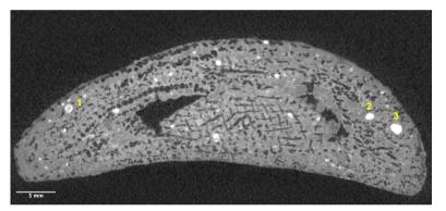
**Figure 6.** Slice from micro-CT of CQ1-13-6 showing inclusions of various sizes and densities throughout. Some of the largest inclusions measure 1.04 mm (1), 1.02 mm (2), and 1.42 mm (3). Some inclusions are biological objects such as seeds (1) while others are very dense and are likely small pebbles.
