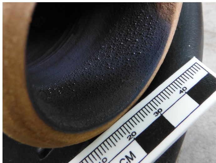
Figure 11. Mercury droplets in black mercury-rich residue along rim of ceramic retort. The blackened interior of a mercury smelter chimney at Karaburun, Türkiye had >400 ppm Hg (Brooks et al., 2017). At the retorts at New Almaden this black sooty residue was scraped and removed to obtain additional mercury (Boulland & Boudreault, 2006).
