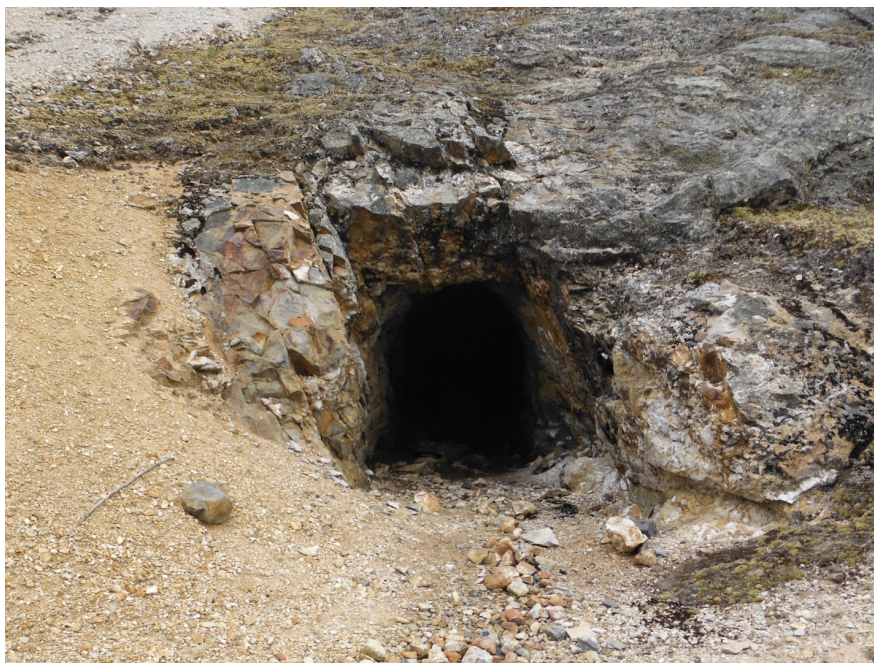
Figure 3. One of several adits at Chonta, note high-angle structure at entry.
